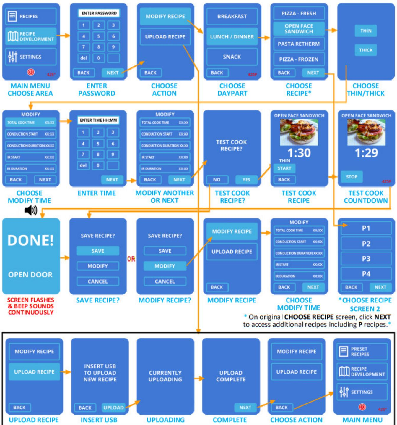
After Upload has been completed, the screen will transition to the main **MODIFY RECIPE / UPLOAD RECIPE** screen after 20 seconds, or the user can select the **NEXT** button.
