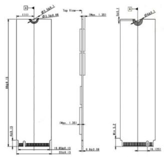
Note: the top side thickness is without the heat spreader. Heat spreader adds approximately 0.4mm to the thickness.
