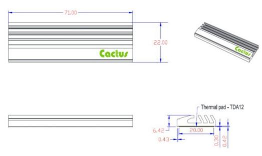
M.2 2280 SSD Heat Sink Dimensions (for extended temp. version)
