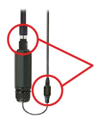
2. Once the antenna is securely screwed onto the CC DX Mile, use the supplied coaxial seal to completely cover the connection. We also recommend coating the USB connection with silicone grease and wrapping with the
