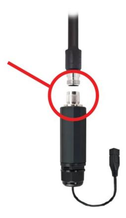
1. Before connecting the CC DX Mile to the antenna, coat the threads of the antenna with the supplied silicone grease. This will help protect the threads from rust and water incursion.
