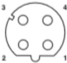
Illustration 10: Pin assignment M12, 4-pin, D-coded, view socket side
