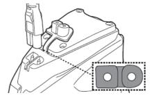
3. Connect the external adaptor to the power source. The indicator light on the external adaptor turns red once the charging begins. The indicator light on the external adaptor will turn green when the robot is charged.
