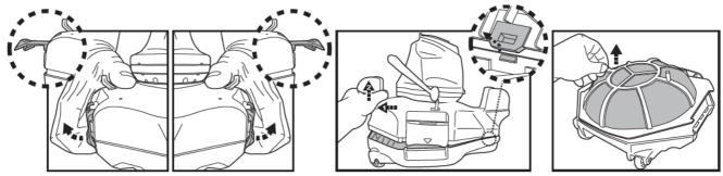
2. Detach the filter cover and remove the debris from the compartment. It is recommended to clean the filter
