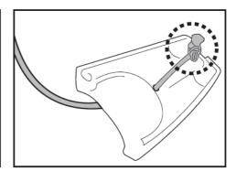
• Replace a damaged flap immediately with a new one before the next operation.
