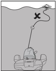
First, align and attach the retrieval cord to the side notches at the top as you wrap the cord around the stem ( step 1 & 2).
