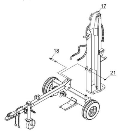
STEP 3: Attach the Beam Assembly
