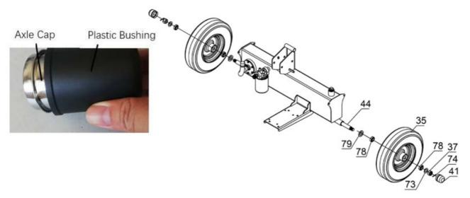
Tips: Use a black plastic bushing to fix the axle cap (#41), cover the black bushing on the axle cap, then use a rubber / wooden hammer to knock the end of the plastic bushing and attach the axle cap onto the wheel.
