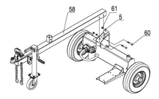
STEP 3: Assemble Beam and Tow Bar and Hydraulic Hose
