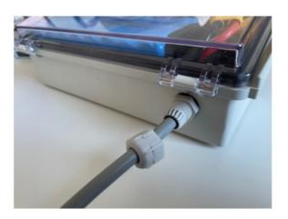
It is important to check the tightness of the cable gland before/at each use. If the cable is compressed, the nut may need to be retightened. It should not be possible to push the cable in or out with the correct pressure of the nut. A loose cable gland can cause water to get inside the battery box and damage and corrode the components inside.
