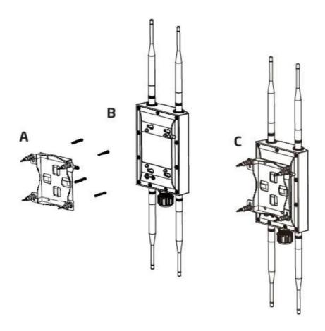
\*The installation angle of antenna must be vertical to the ground.
