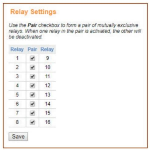
Click the Pair checkbox in the center column to pair the associated relays (1 and 9, 2, and 10, etc.). When paired, the relays will behave as one raise/lower channel. When not paired, each relay behaves independently.
