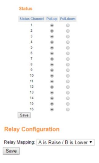
Each status input on the Plus-X GSC Adapter can be configured as pullup or pull-down. To configure the status channels, use the Status Configuration link on the Plus-X GSC Adapter's web page. For each channel, select either Pull-up or Pull-down. Click Save when you are finished.
