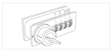
6. Turn the knob to the open position (arrow points to the to the green lock symbol) and pull the door open. Remove the master key. To lock, follow step 1 under the point "Operation".
