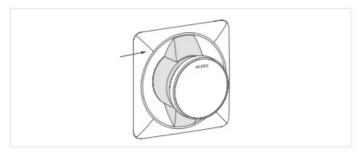
2. Carefully insert the opening pin into the closure hole underneath the operating panel until resistance is reached and press lightly.
