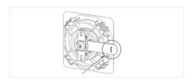
2. If the electronic lock is installed in the European Economic Community (EU and EFTA), the enclosed type plate must be clearly visible, legible and permanently affixed to the cam (on the back of the door). Otherwise the product does not comply with the safety standard of the RED (Radio Equipment Directive).
