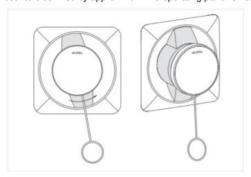
4. Remove the opening pin and pull the operating panel forwards.
