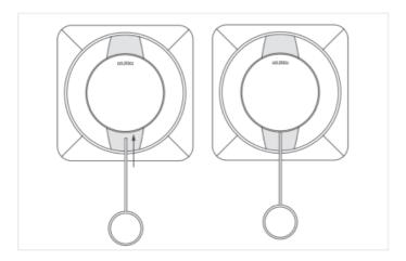
3. Hold the opening pin in position and turn the pin with the housing (shown as a gray area in the sketch) counterclockwise by approx. 10°. The operating panel is not rotated during this process.
