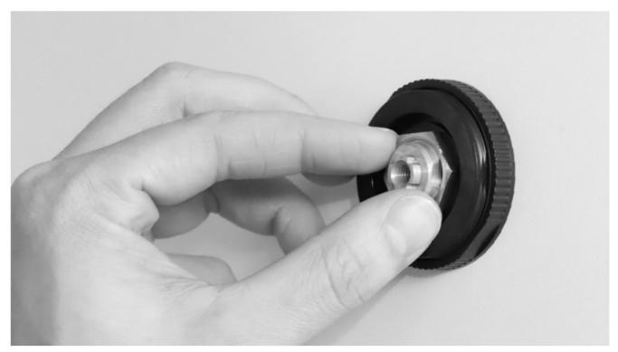
5. Place the latch and fasten it with the Torx screw (Torx 30) provided.
