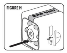
**Night Mode** -When Cop Cam-is an and motion is detected, it will continue to record even in darkness. Infrared lights around the camera's lens (Figure N) will be activated but are not visibly lit
