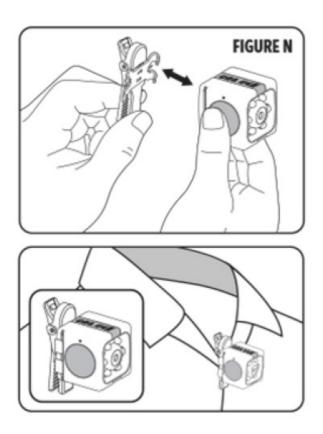
**NO1E:** Clips will make a slight dick sound to indicate proper installation. Make sure POWER/RECORD button & charging port are oriented on the left and right side of the unit when in use. To remove the swivel dip, gently slide the dips either up or down out of the camera mounting grooves.
