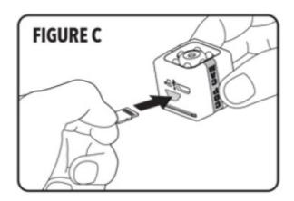
**STEP 3:** To retrieve footage, remove memory card by pressing inward to release, then pull out of slot. (Figure C) Use included USB cable to connect Cop Cam" to your Computer/Laptop. Access footage following prompts. (Figure D)
