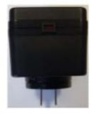
The RF Beacon is a plug-based device that is inserted into a fixed mains socket, to provide a location reference for the Smart Tag equipment. The device is available in different pin configurations to allow for direct connection to the mains supply in the country of use, without the need for an adaptor.
