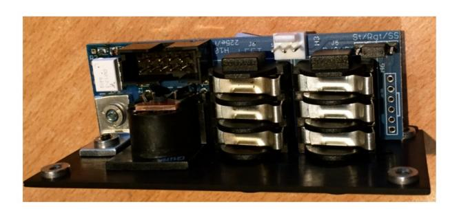
If the jumper was in the "St" [Stereo] position (connecting pins 3 and 4) then the left audio jack becomes a Stereo output.
