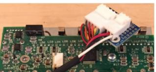
For use with a 207e or 206e, you replace the 5pin audio output cable with this little board as pictured. Restore the audio to the panel by inserting the 207e or 206e audio cable back in to the right angle 5pin header and then insert a 3pin cable into the 3pin header and plug the other end into the 22X-I-O.
