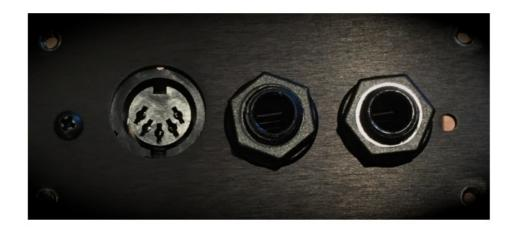
For use with a 225e (or 225h), use the 10pin header to connect the 5-pin DIN MIDI input.
