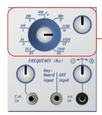
The **Modulation oscillator's frequency knob** adjusts semitones, and the smaller knobs handle **detuning**. To play the note center pitch, set both the fine-tune and the large knob to the minimum.
