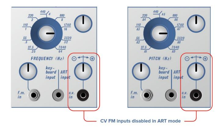
To demonstrate the use of ART, we will use Tiptop Audio's Octopus ART module, though any other module that outputs ART, such as ART V/OCT, Model 264t, etc., can be used in the same manner. To activate the Autotuning for the first time, the module needs to learn the environment it is in, this process is called INITIAL TUNING.
