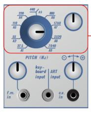
The **Principal oscillator's frequency knob** adjusts **octaves**, while the smaller knob handles fine up-tuning. To play the note center pitch, set only the fine-tune knob to the minimum.
