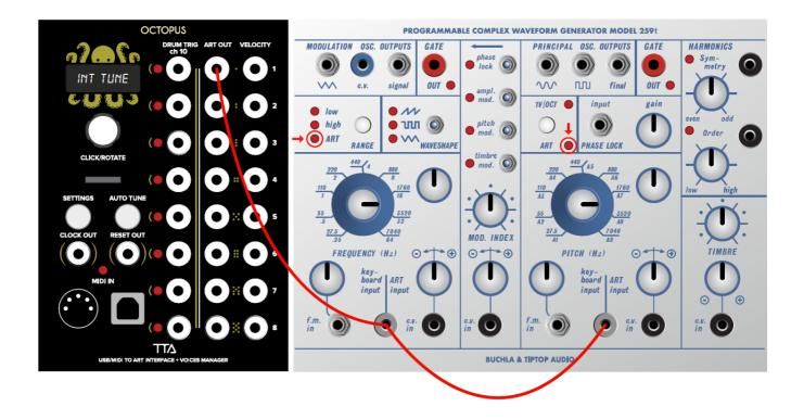
In this patch we demonstrate the use of the ART V/OCT module to quantize 245t CV steps into ART notes for the 259t.
