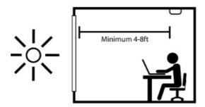
· Check that the daylight sensor's view is not obscured.
