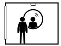
• The sensor should be place 4 to 8 feet away from the window (or 2 times the height of the window)
