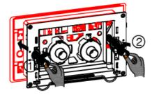
15. Once the toilet is installed and the front panel secured, fit the flush panel control.
