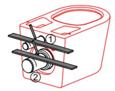
5. Check both pipes to ensure they are the correct length.
