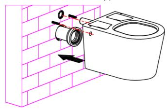
12. Check for level and tighten bolts.
