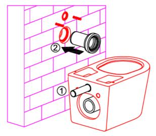
11. Secure the toilet pan onto the studs and connect the waste pipes.
