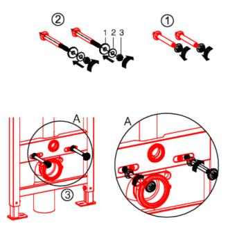
6. Position the frame within the cabinet and mark up the appropriate fixing points ready for drilling and screwing.
