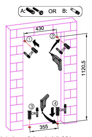
8. Secure the frame kit into the cabinet using supplied securing bolts & fixings.
