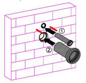
2. Measure the pipe lengths required and mark accordingly.
