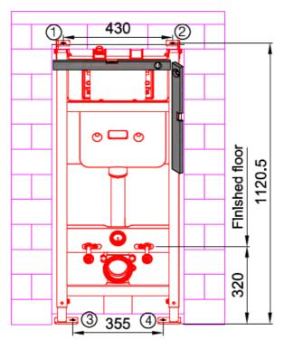
7. Using appropriately sized drill bits & screws, secure the cabinet in your chosen location.
