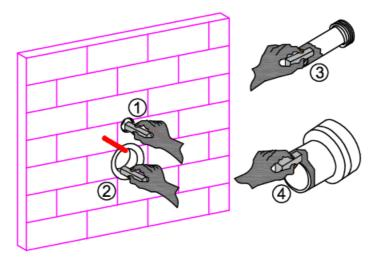
9. As per the illustration, measure the size of d. Hang the toilet to the 2 screw bolts which need to be 25mm longer than the size of d.
