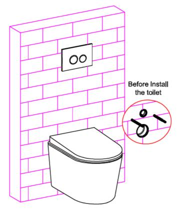
1. Insert both the soil & flush pipes into the joints.
