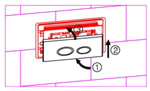
16. Disassembly: As per illustration, push the button plate upward and then pull it out as per illustration 2.
