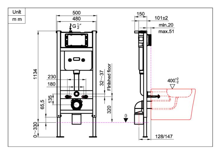
1. Assemble the fixation frame to the tank in the correct position, As in Picture 1
