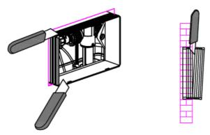
12. Loosen the angle valve, and connect the inlet pipe to the angle valve. Anale valve diameter: G1/2
