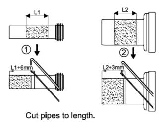
7. Using a file, chamfer the end of the pipes to enable ease of installation into the sockets.
