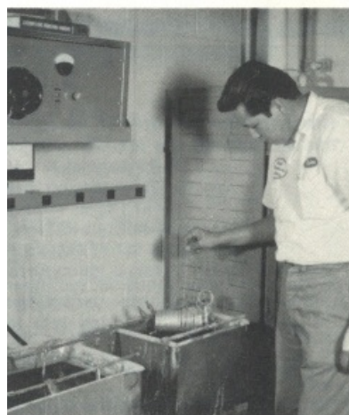
Radio Band Switch Deck and Tank Coil assembly is Silver Plated after soldering.
