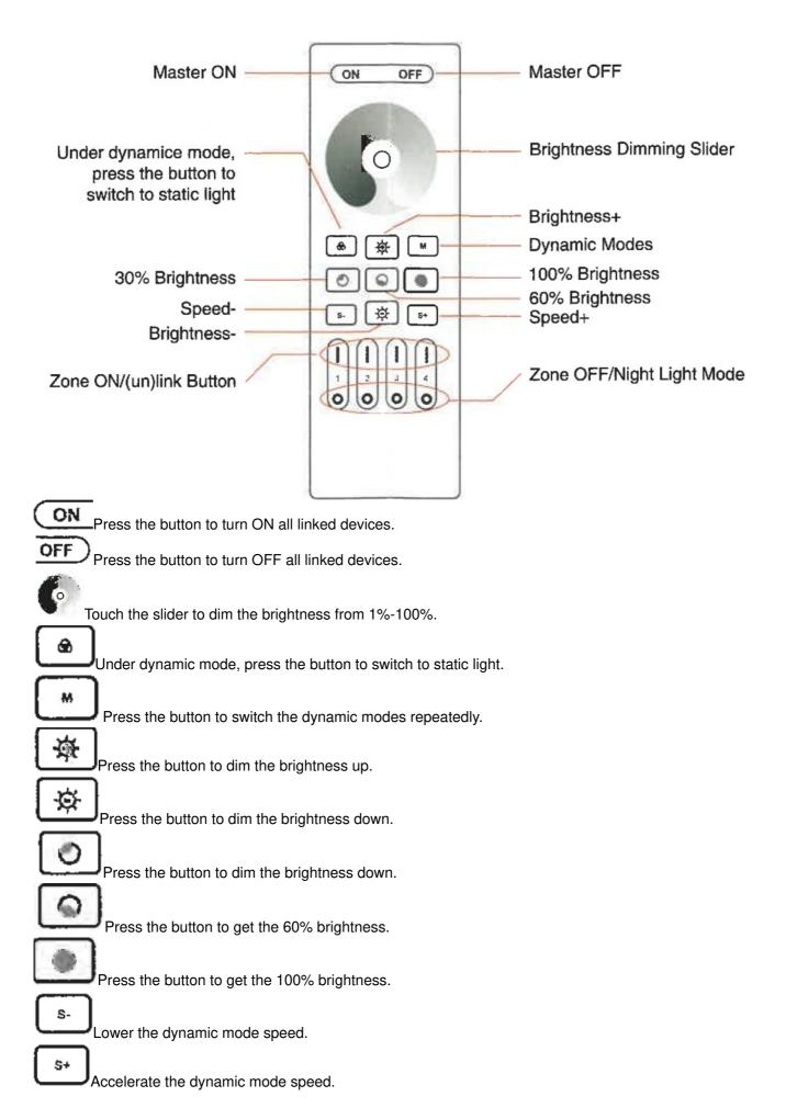
RC02RF/RC02RFB: 4-Zone DIM&CCT Remote Control
