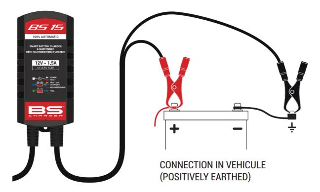
If Positively Earthed – FIRST Connect the Black (-) battery charger lead to the Negative (-) battery post and then connect the Red (+) battery charger lead to the Vehicle's chassis and far away from the fuel line.
