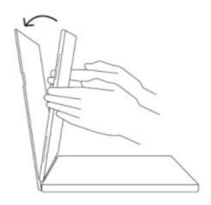
**TO REMOVE:** Place your Brydge on a flat surface. Use the tabs on either side of the case to release the iPad.
