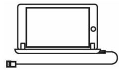
• The battery is charging when the light on the power key is red; your Brydge is fully charged when the light turns off Once done charging you can remove the cable (battery should last 12 months or more based on use)
