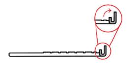
**TO INSERT:** Insert your iPad (in a protective case) into the hinges with the home button on the left.
