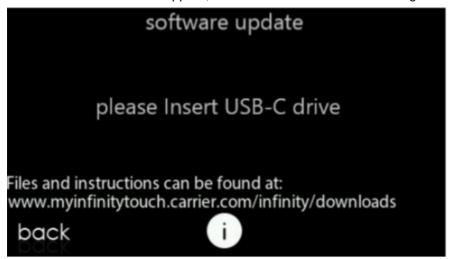
• If the .bex file is stored properly on the USB-C drive, this screen will appear. If the screen says, "Please insert USB-C drive", remove the USB-C drive and re-insert. If it still does not show the screen, below, go back to the download part and retry.
