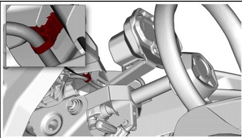
**4. Apply pressure on the FDM module [P1] to clip it on the FDM support [P3].**
