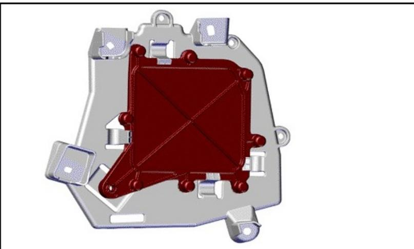
**5. Install the FDM support [P3] with four PT type K-50 x 16 Screw [P8].**
