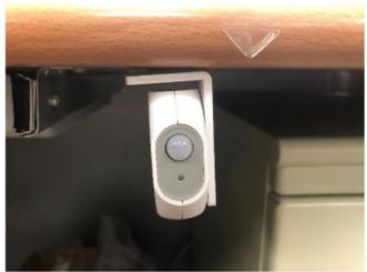
**Step 5**Adjust to the desired angle and stick the sensor on the bracket. Avoid covering the QR code.
