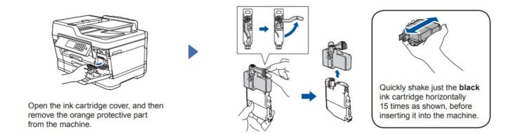
Follow the Touchscreen instructions to unpack and install the ink cartridges The machine will prepare the ink tube system for printing
