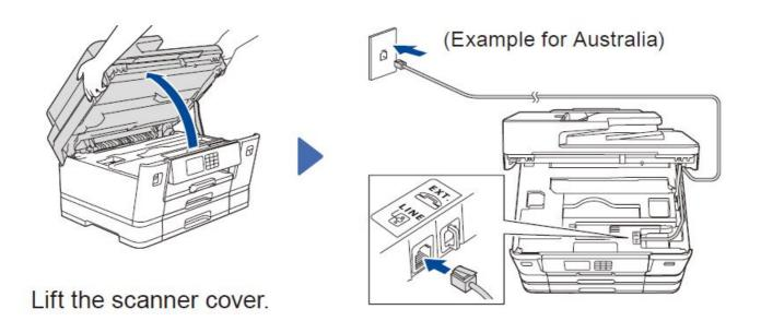
Connect the telephone line cord. Use the socket marked LINE and guide the cord out the back of the machine.
