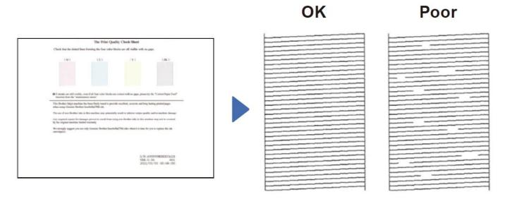
Follow the LCD instructions and check the quality of the four colour blocks on the sheet, and then start the cleaning procedure if required.
