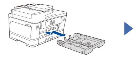
Pull the paper tray completely out of the machine as shown by the arrow.
