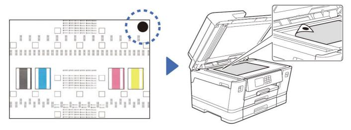
Follow the LCD instructions to print the Adjustment Sheet. The black circle mark is located in the upper right corner of the sheet. Place the Adjustment Sheet face down on the scanner glass. Make sure the black circle is in the upper left corner of the scanner glass.
