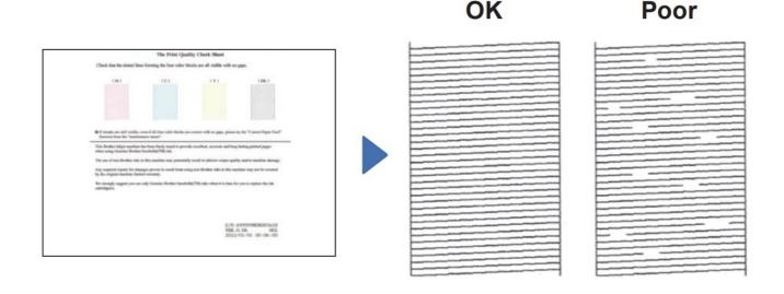
Follow the LCD instructions and check the quality of the four color blocks on the sheet, and then start the cleaning procedure if required.
