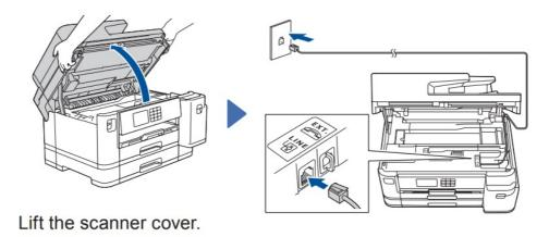
Connect the telephone line cord. Use the jack marked LINE and guide the cord out the back of the machine.
