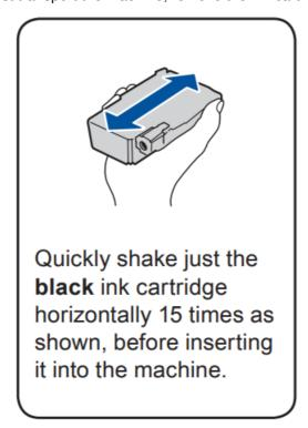
Follow the LCD instructions to install the ink cartridges. Close the ink cartridge cover. The machine will prepare the ink tube system for printing.
