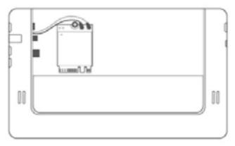
3. Gently disconnect the antenna connectors, then loosen and take out the existing M.2 network adapter from your laptop's motherboard.
