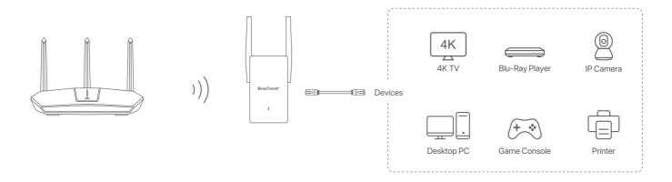
In this case, you need to configure the IP Address and DNS server address of these devices as AUTO OBTAIN.
