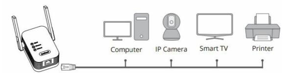
2. For optimal connection for your wired device, we do not recommend connecting other Wi-Fi devices to the extended networks created by this adapter, which may lower the speed of your wired device. You can log back into the web management page of this adapter to turn off the extended network.
