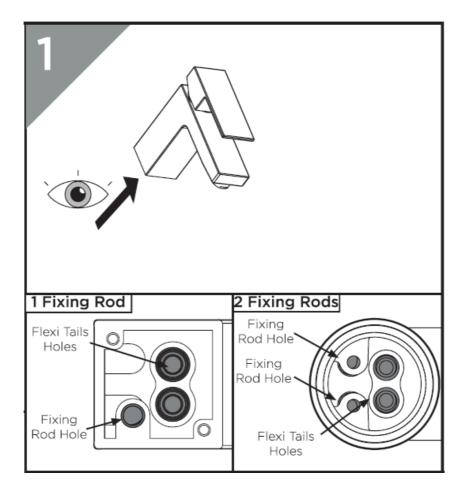
• Screw in the fixing kit rod(s) into the base of the tap with a screwdriver
