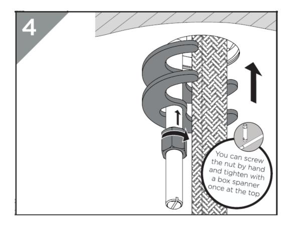
• Connect the hot and cold water supplies to the flexible tails and turn until tight
