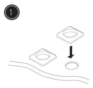
Place the plinths over the holes in the basin ensuring that the washers are fitted between the plinths and the basin/ bath.
