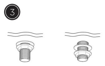
Secure the tap bodies to the basin/bath by using the washer and metal backnut below the basin /bath. Tighten the backnut onto the thread ed tails. A suitable spanner may be required to fully tighten the backnut.
