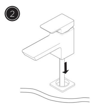
Place the plinth over the hole in the basin/ bath and feed the flexi tails through.
