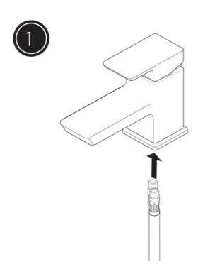
Screw the flexi/copper tails into the bottom of the tap body by hand only (DO NOT OVERTIGHTEN).
