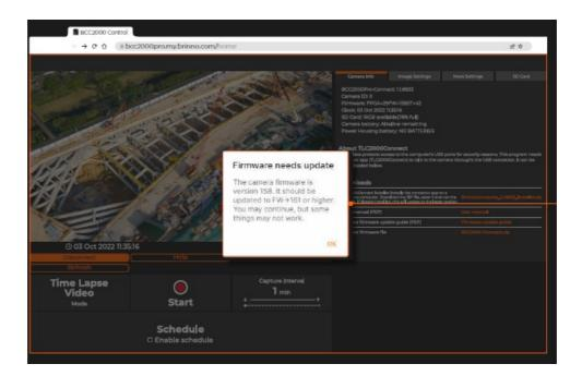
While using an Internet connection, the online Brinno Command Center will detect whether the camera's firmware is the latest version. If it's not, there will be a pop up notification to tell you to update your firmware. Go to the TLC2000/TLC2020 support page and download firmware in your desired language.
