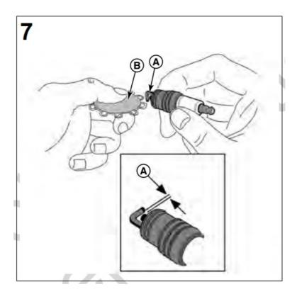
Check the gap (A, Figure 7) with a wire gauge (B). If necessary, reset the gap. Install and tighten the spark plug to the recommended torque. For gap setting or torque, see the Specifications section.
