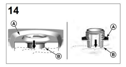
Store the engine level (normal operating position). Fill fuel tank (A, Figure 14) with fuel. To allow for expansion of fuel, do not overfill above the fuel tank neck (B).
