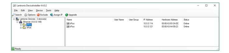
Device Installer will show all devices located on your network. To identify the correct device from its Serial Number, double-click a device with the name "xPico". This will show a Device Info tab. Use the DHCP Device Name property value to determine if this is the correct device.
