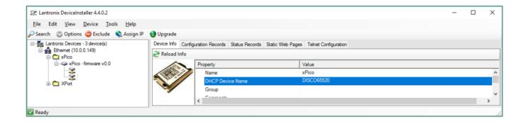
Having determined the correct device, note the IP Address assigned to it and open a web browser to that address, for example http://10.0.0.121. When prompted for a username and password, leave both fields blank and click OK.
