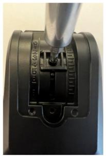
3. Step 3 This will now allow the lens to slide up and down to find the desired viewing angle. Once the camera has been adjusted to the desired angle, tighten the screw on the sliding mechanism, then replace cover and fixing screw.
