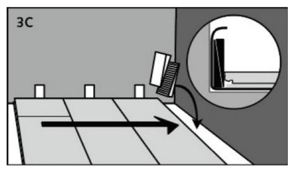
The diagrams indicate where the Uniclic panels are clicked together by angling up and down or where they are tapped together flat. Follow the diagrams precisely. See diagrams 4.1 > 4.16
