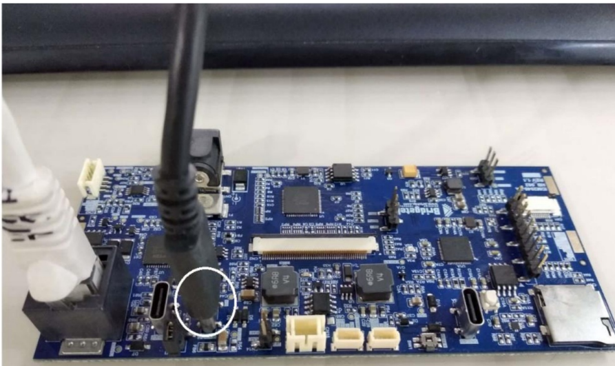
e. Turn on the 20v adapter using the AC power supply.
