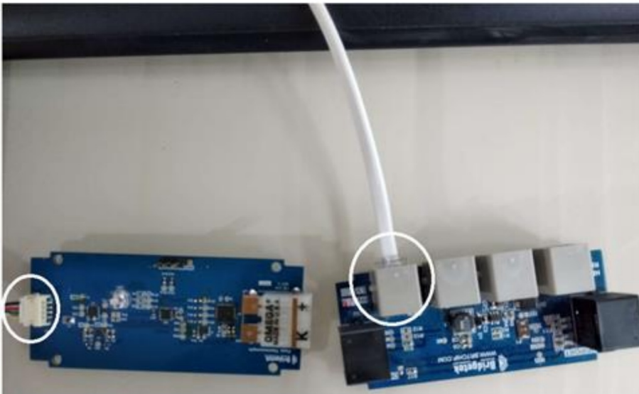
c. Using RJ45 cable, connect HVT to IDM2040 RJ45 connector.
