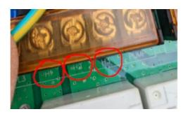
These three terminals are connected to the three active sides of the three heating elements. Remove the jumper cables that bridge H1, H2 and H3 together.'
