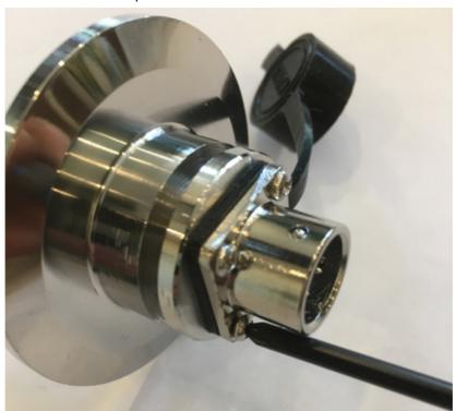
3. Gently slide the sensor out and inspect the wire joints at the connector end and at the sensor end. An unconnected wire will cause the sensor to malfunction. The compound on the sensor is a heat transfer compound and should not be removed as it facilitates faster temperature reading.
