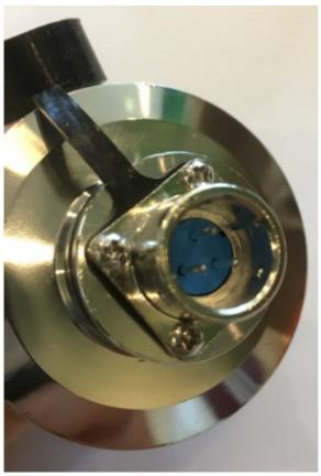
2. Loosen the four screws with a small Phillips screwdriver.
