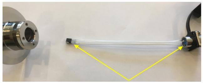
4. The sensor is a small computer chip and should be treated carefully as one would a computer (ie. don't be rough with it and don't place it near a magnet).
