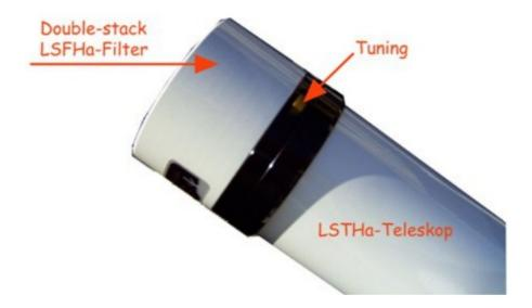
It can happen that you will see the following picture in your eyepiece, after you have your double-stack filter screwed on. Then you just have to tune your double-stack filter to move the sun reflexes out of your field of view.
