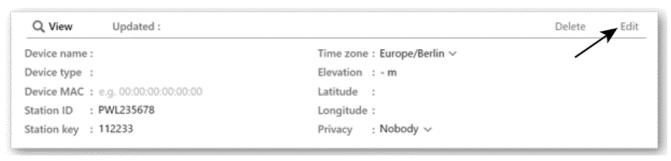
5. Enter the "Device name", "Device MAC address", "Elevation", "Latitude", "Longitude" and select your time zone in the station tab, then click "Confirm " to save the setting.
