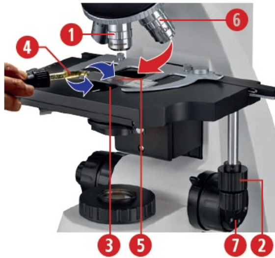
Fig. 10: Using the 100x oil immersion objective.
