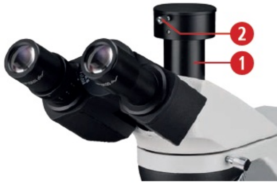
Fig. 7: Trino tube for the photography.
