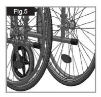
Step tubes are used by attendants to tip a wheelchair over an obstacle. Simply step on the tube to push a wheelchair, for example, over a kerb or step.
