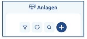
2. Register, log in, and click the plus symbol to set up a new plant. An internet connection is required for this.
